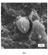
**Figure 1** SEM fractography of impact fracture surface of (a) A/B/MBS 50/50/5 and (b) A/B/PMMA/MBS 45/45/10/5.
