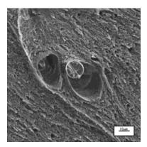
**Figure 2** SEM fractography of impact fracture surface of A/B/PMMA/PA/SMA8/MBS 40/40/10/10/2/5 shows unbonded glass fibers in channel-like holes.
